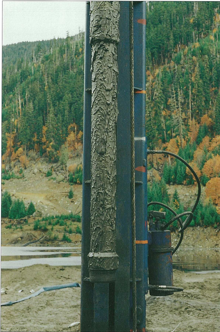
Photograph 6. Myra Falls tailings adhering to Vibro-Drain extension rod after withdrawal from ground
